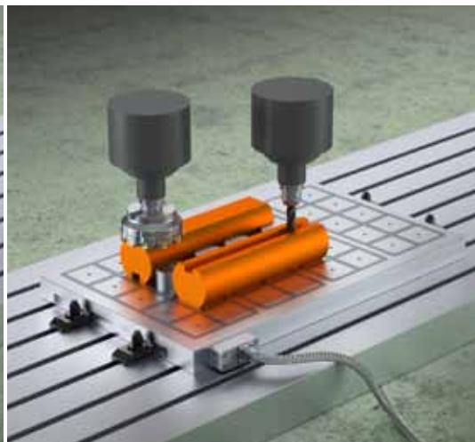
Round bar facing and slots milling
